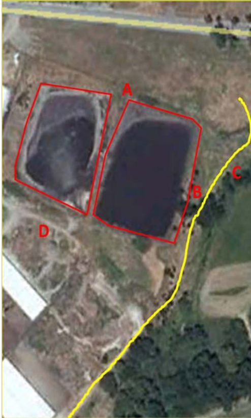
Figure 1-1. Current manure lagoons serving the free stall milking cow barn. Manure from the production area is flushed and placed into the two manure lagoons (A). Overtopping of manure slurry from the lagoons contributes to nutrient loading to Windsor Creek at point (B). An interim berm (C) will be placed along the ridge located above Windsor Creek to protect against manure-related nutrient loading. The solids will be stacked and dewatered adjacent to the existing manure separated solids piles (D). The interim berm will serve to protect the Creek from nutrient loading from both the overtopping of lagoons and runoff from the separated solids stacking pile. (Photo Credit: Google Earth)
